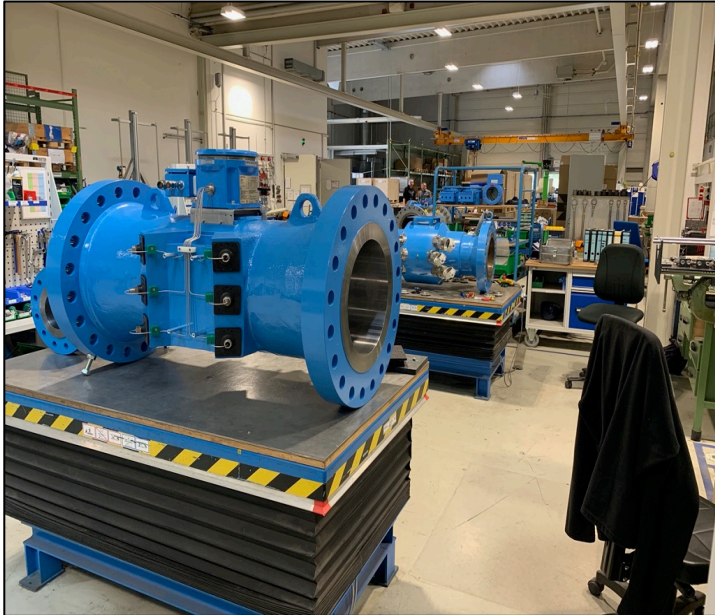
Figure 1 – Meter Assembly Table
