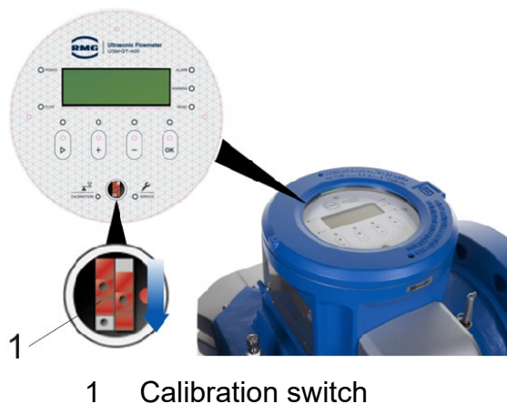
Fig. 10.7: Close the calibration switch
