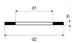
Dimensions of the seal: d1 = Inside diameter d2 = Outside diameter
