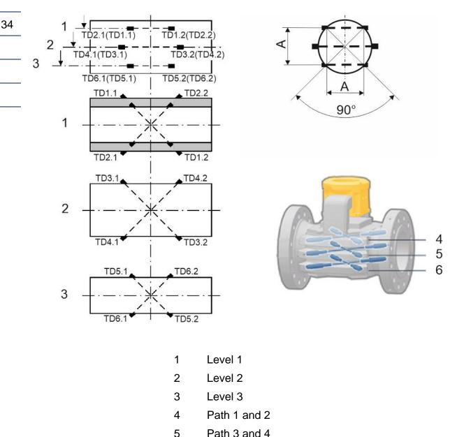
Fig. 3.5: Transducer paths and levels of the ultrasconic gas meter
