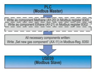
Fig. 4.6: Import of data via Modbus
