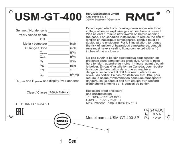
Fig. 13.7: Position of the official seal on the type plate
