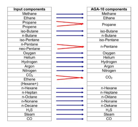
Fig. 4.8: Classification of gas components
