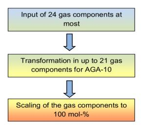
Fig. 4.7: Sequence of gas components treatments
