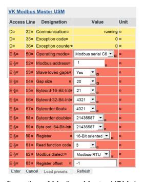
Fig. 8.27: Configuration of Modbus Master USM due to Instanz-F
