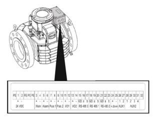
Fig. 8.5: Connection assignment on the terminal strip
