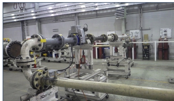
Double Elbow Out-of-Plane (DEOOP) Testing
