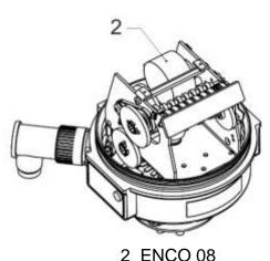
Figure 3: Type "F" meter head
