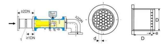
1 Perforated Plate Straightener
