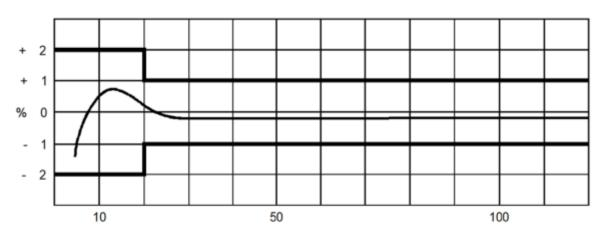
Figure 2: Calibration curve of a turbine meter
