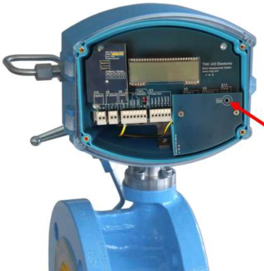
Figure 8: Position of the calibration button
