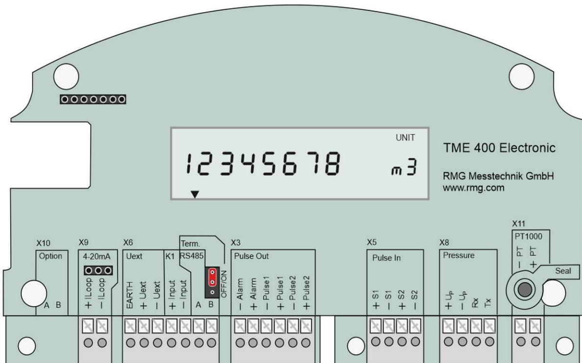
**Figure 5: Connection assignment of the TME 400**
