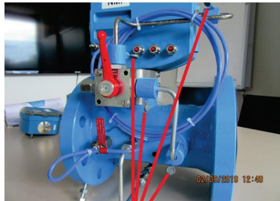
Seal cap with lead seal
