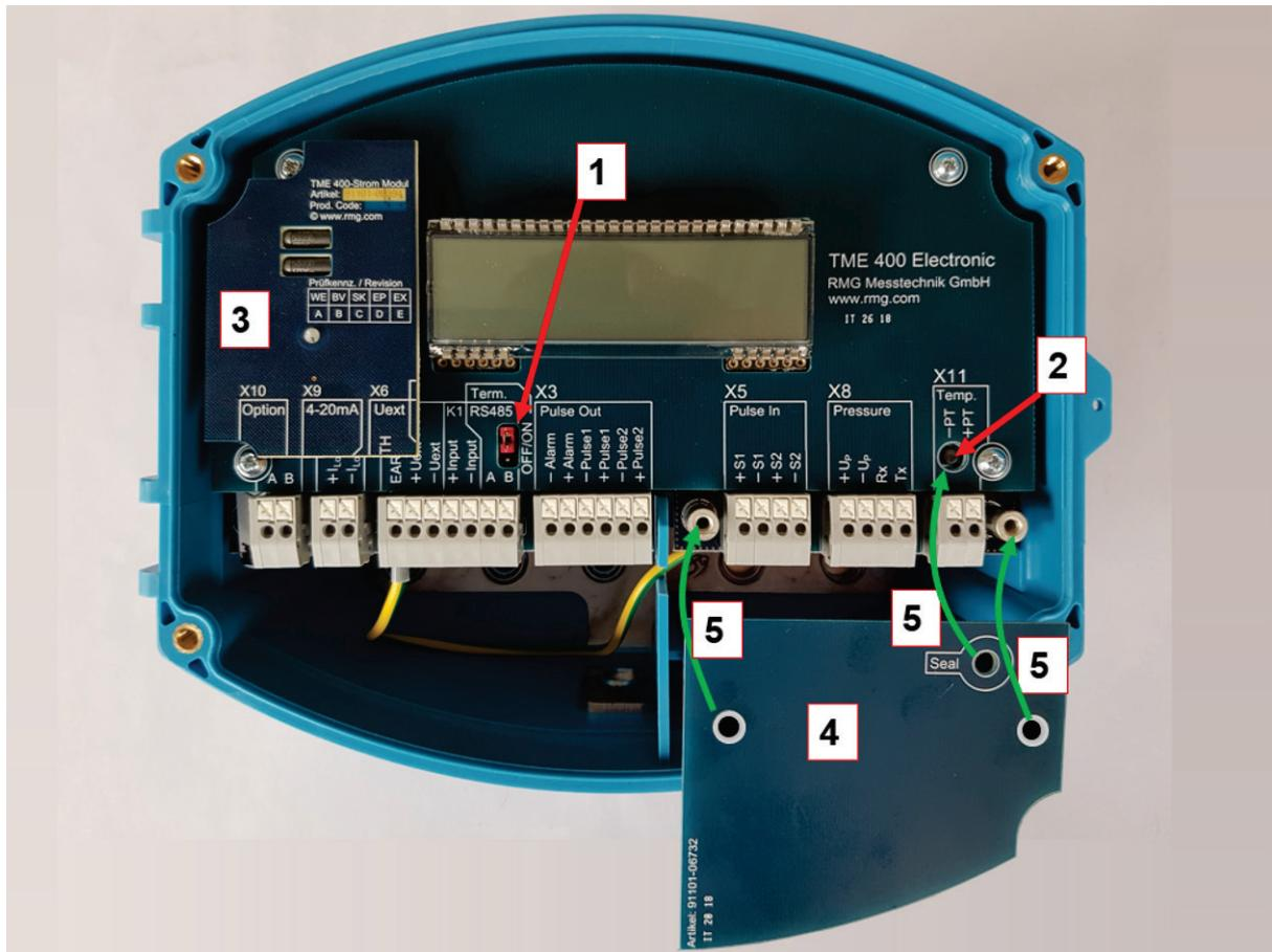
**Figure 4: Electronics with cover of the calibration button**
