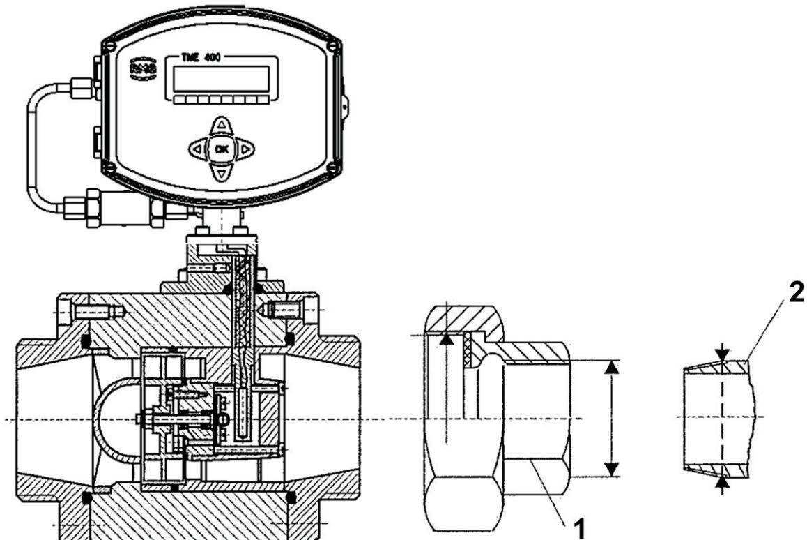
**Figure 2: Threaded connection for DN25 and DN40**
