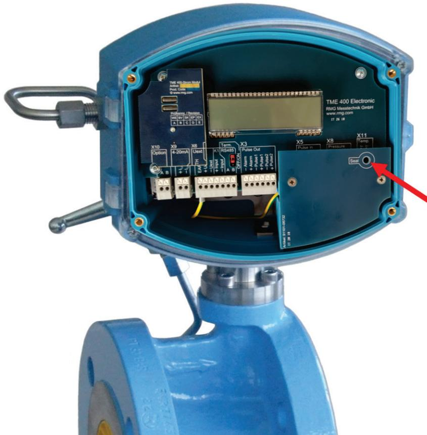
*Figure 8: Position of the calibration button*
