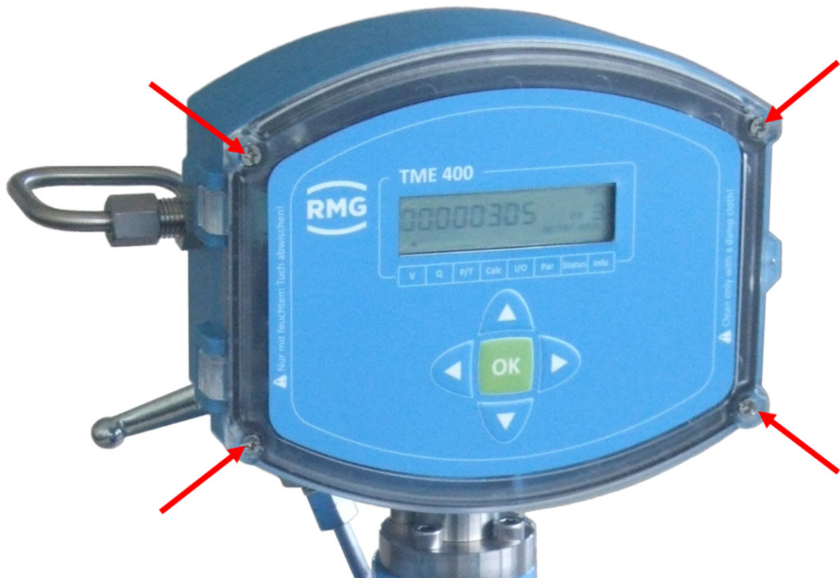
Figure 3: Unscrewing the screws to open the cover
