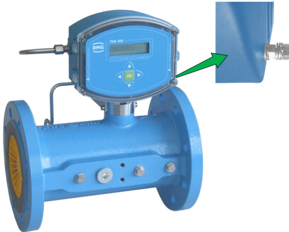
Figure 16: Grounding the meter
