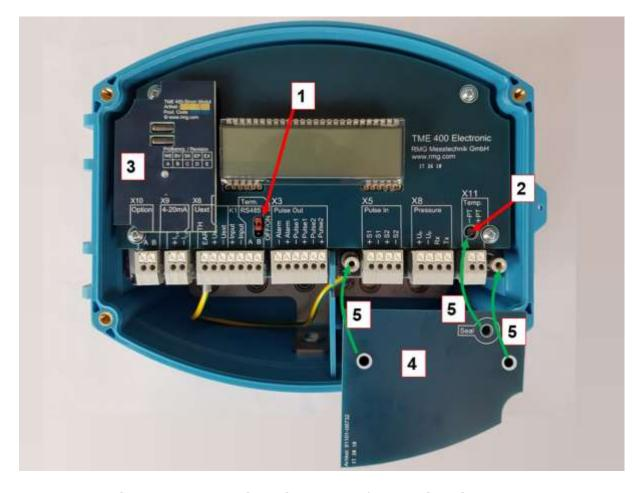
Figure 4: Electronics with cover of the calibration button
