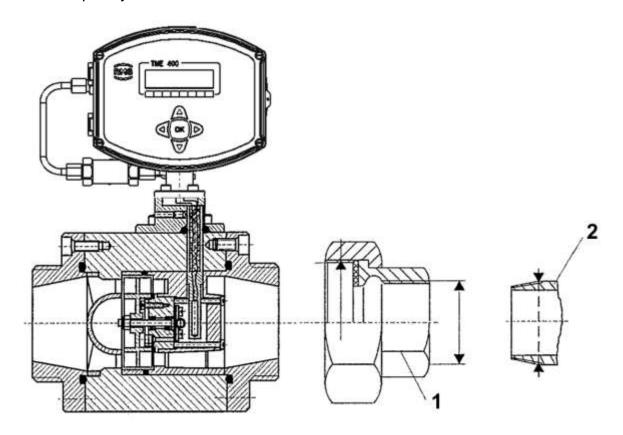
Figure 2: Threaded connection for DN25 and DN40
