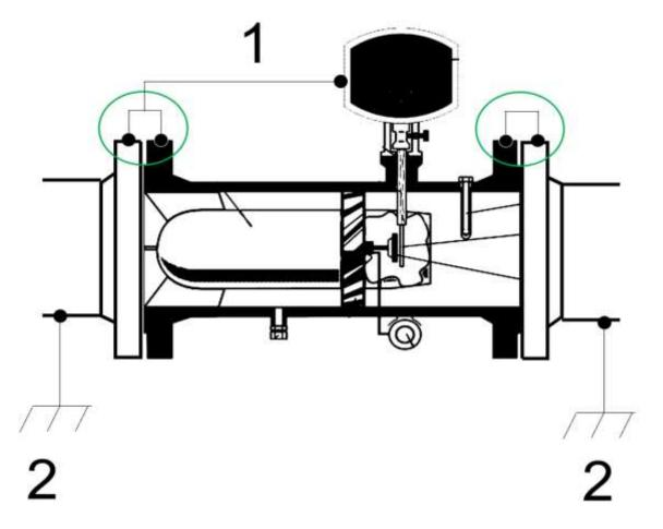
Figure 17: Grounding with the connecting pipes
