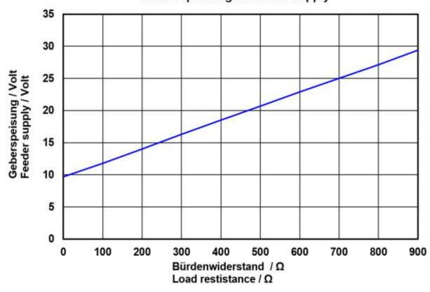
Figure 14: Load depending on feeder supply
