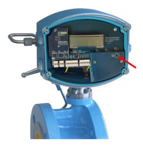
Figure 8: Position of the calibration button
