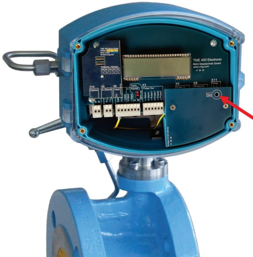
**Figure 8: Position of the calibration button**
