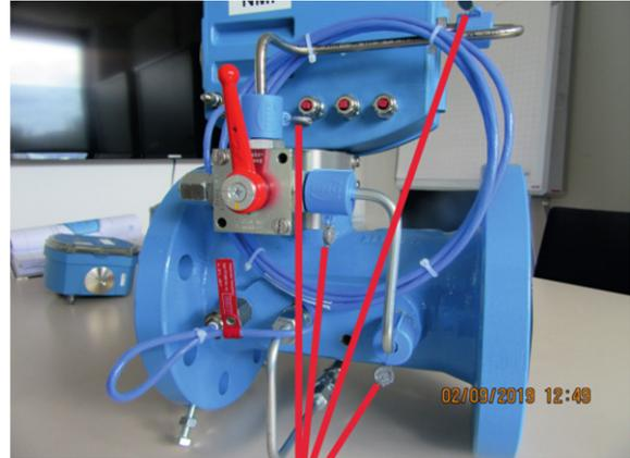
Seal cap with lead seal
