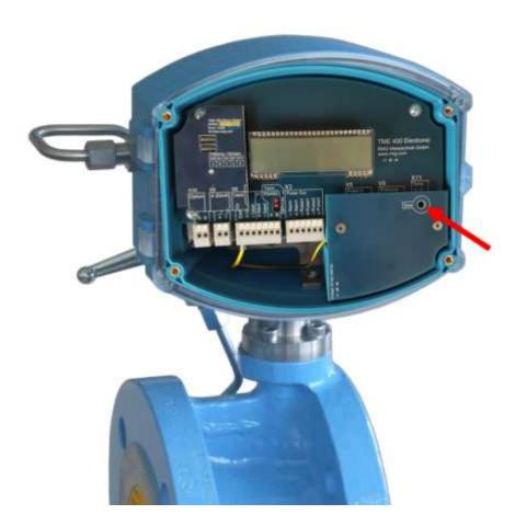
Figure 8: Position of the calibration button
