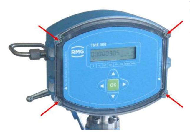
Figure 3: Unscrewing the screws to open the cover
