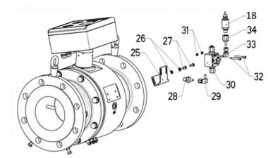
Figure 68: Version with 3-way valve with pressure transducer
