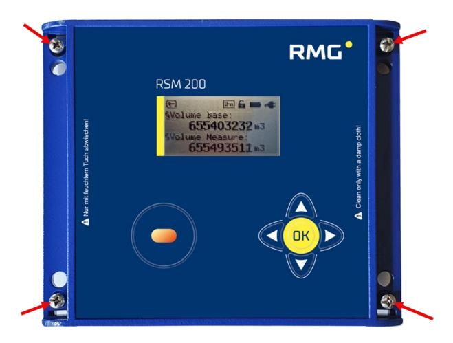
Figure 9: Unscrewing the screws to open the cover
