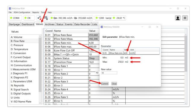
Figure 45: Change of parameters via RMGView<sup>RSM</sup>
