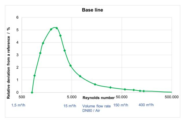
Figure 5: Typical basic characteristic curve
