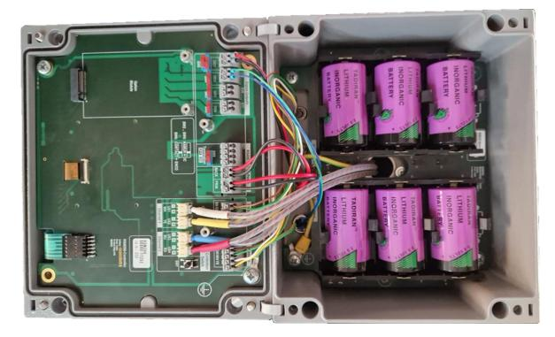
Figure 17: Location of the battery compartment
