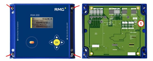
Figure 16: Position of the calibration switch
