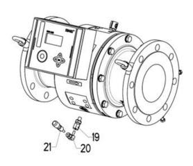
Figure 66: Version pressure connection Ø 6 mm and mini measuring coupling
