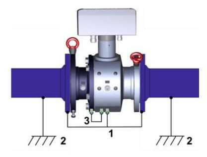
Figure 14: Grounding with the connecting pipes
