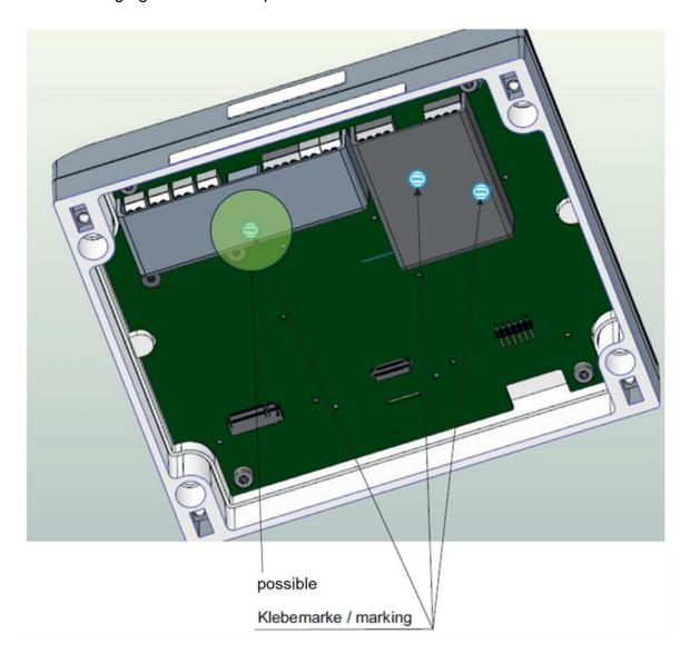
Figure 61: Seals in the inner of RSM 200
