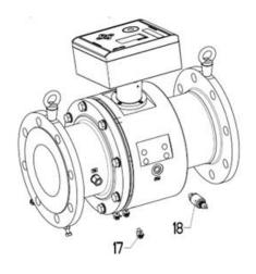
Figure 64: General version with pressure transducer
