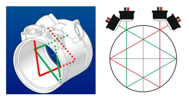
Figure 4: Double reflection of the ultrasonic beams
