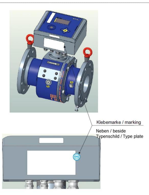
Figure 62: Seals at the electronic housing of RSM 200
