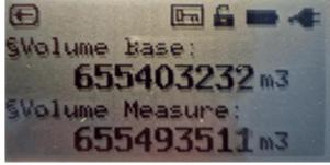
Figure 31: Main/start display (without / with quantity transformer)
