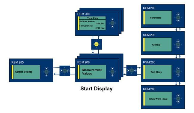
Figure 29: Display settings and operation
