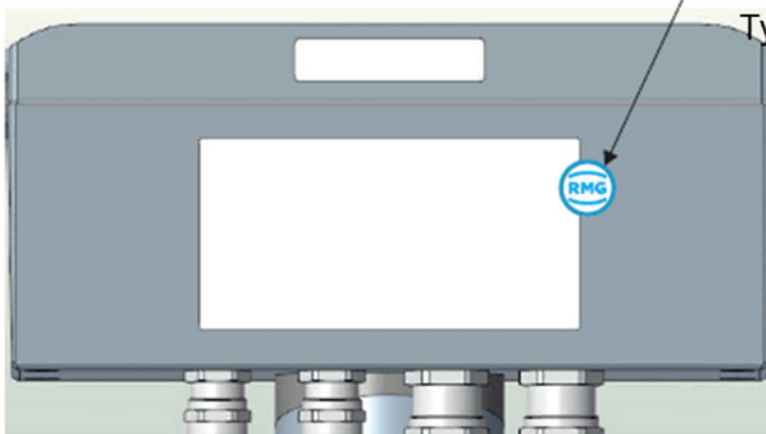
Figure 66: Seals at the electronic housing of RSM 200
