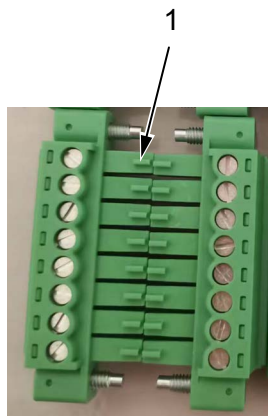
Fig. 20: Strip on connector (Phoenix)
