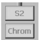
Grey color of the gas stream symbol and gray text mean that the gas stream is not available for the present version.
