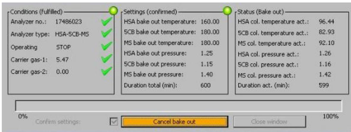
After termination of the heating process, cooling is started immediately. Now no more actions and interventions in the cooling process are possible and the cooling time (always 1 hour) has to be waited.
