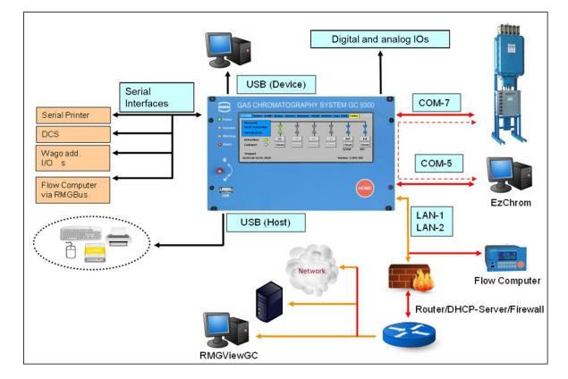
The PGC measurement element is connected via COM 7 and a PC can be connected via COM 5. The LAN 1 and LAN 2 connections allow the connection of an ERZ2000 (ERZ2000-NG or ERZ2000-DI) and the integration into a PC network. Additionally, the RMGView<sup>GC</sup> software can also be activated here, which allows convenient operation of the GC9390. These operating options are described in the corresponding manual of the RMGView<sup>GC</sup> software.
