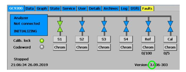
Some further settings are required. In the **menu "Detail"** the COM 7 protocol must be set to CP for the measuring unit (see next figure in the green circle).
