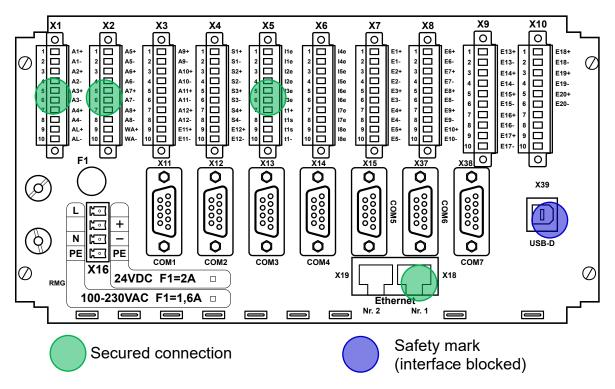
The connections are made on the rear wall. If the number of inputs/outputs is not adequate, an additional module (Wago) with additional digital and analog inputs
