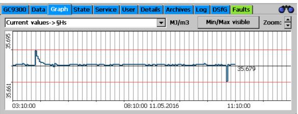
The trends of arbitrary values are displayed the "Graph - Trends" screen. Recording takes place for 60 hours (2.5 days). An interval of 10 hours is always displayed.
