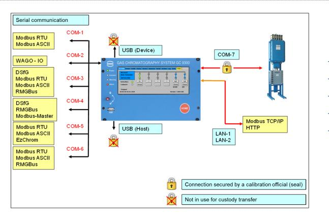
Furthermore, the different protocols are listed, which can be operated at the COM interfaces.
