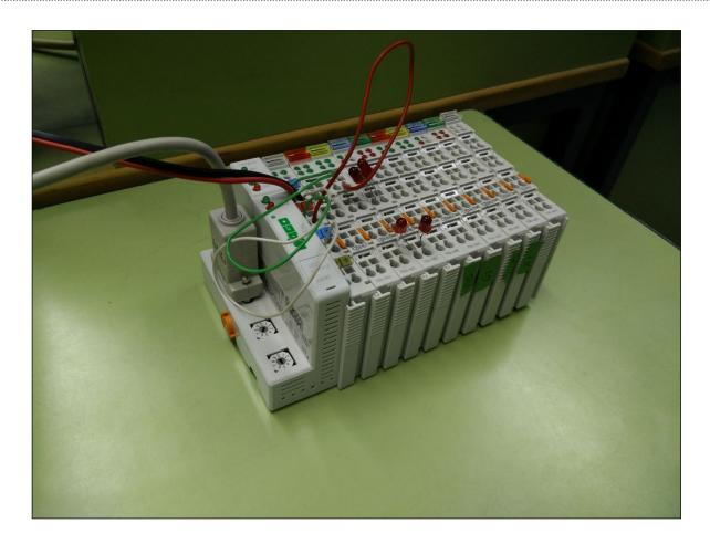
The connection module, the fieldbus coupler as Wago 750-314 or Wago 750-316, as well as the end module, the bus terminal Wago 750-600 are fixed. Between the connection module and the end module you may choose the modules:
