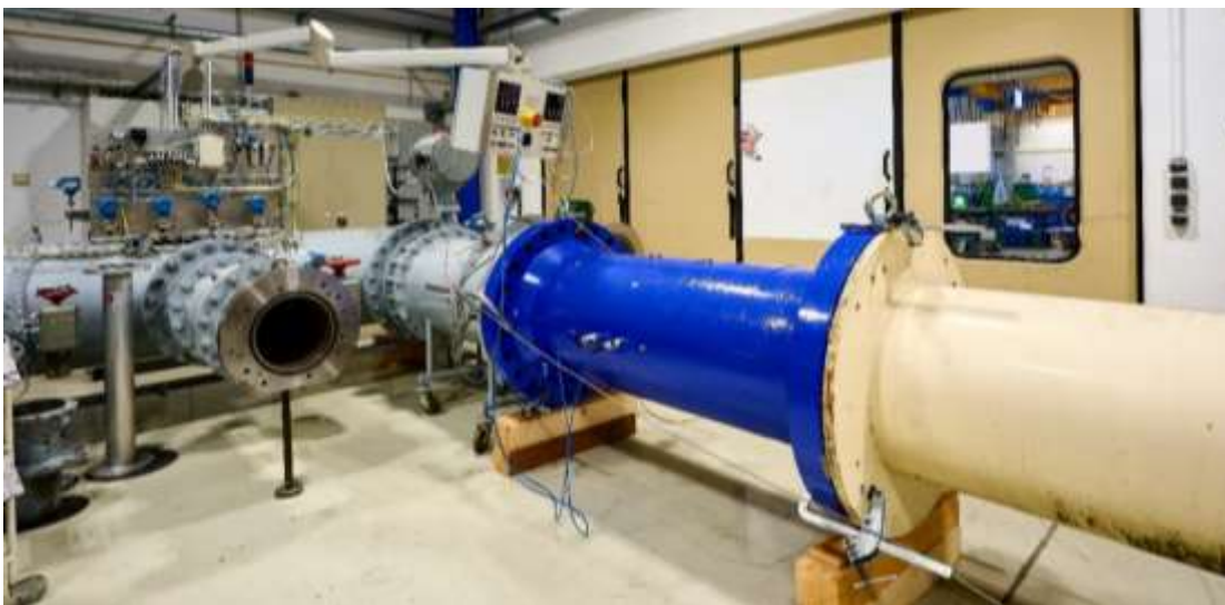
Figure 1 internal calibration of a TRZ 03 DN600 ANSI600RF in Butzbach
