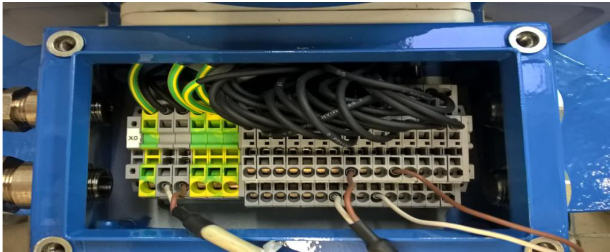
Figure 165: Connection of the RS 485-2 (22 +, 23 -) on the USM GT400
