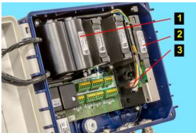
Fig. 26: Connecting the modem battery for Primus 400
