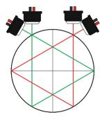
Inside the RSM 200 is the measuring cell with the ultrasonic sensors. In order to determine the velocity averaged over the pipe cross-section, the measuring path is implemented as a Gaussian integration using a double reflection. A second measurement path covers further cross-sectional areas and also records a swirl flow reverse influence on the measurement signal. In total, the influence of a swirl flow is compensated.
