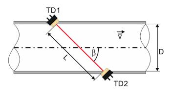
The propagation times of the ultrasonic pulse are determined with the ultrasonic electronics. With tTD12 (running times from TD1 to TD2) and tTD21 (running times from TD2 to TD1) the average speed  $\bar{\nu}$  along the measuring path can be determined.
