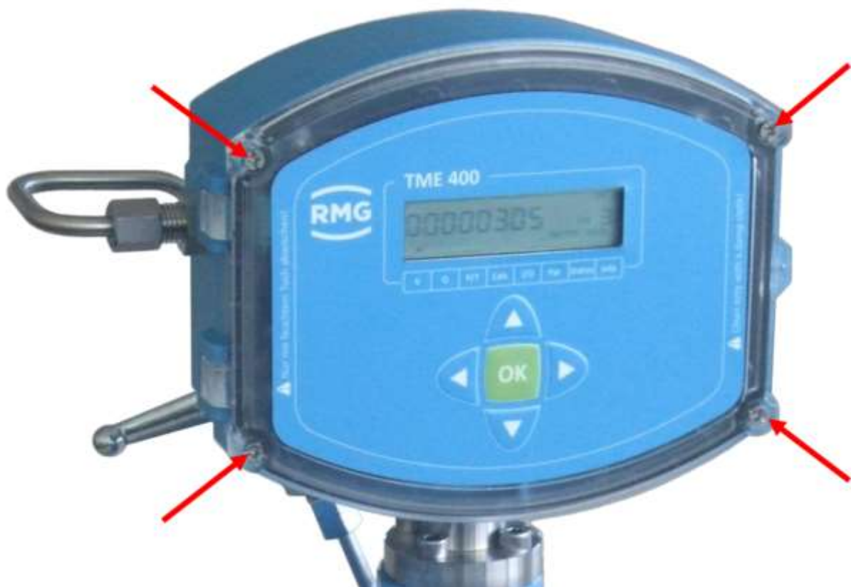
Figure 3: Unscrewing the screws to open the cover
