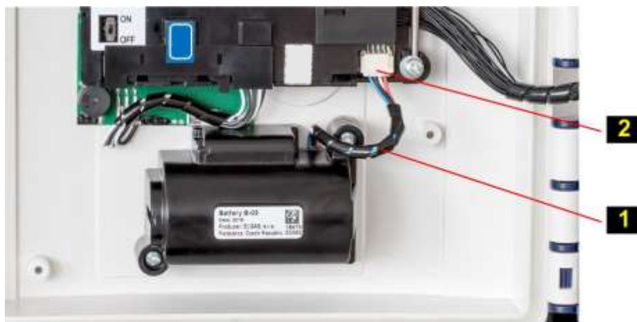
Fig. 25: Connecting the device battery
